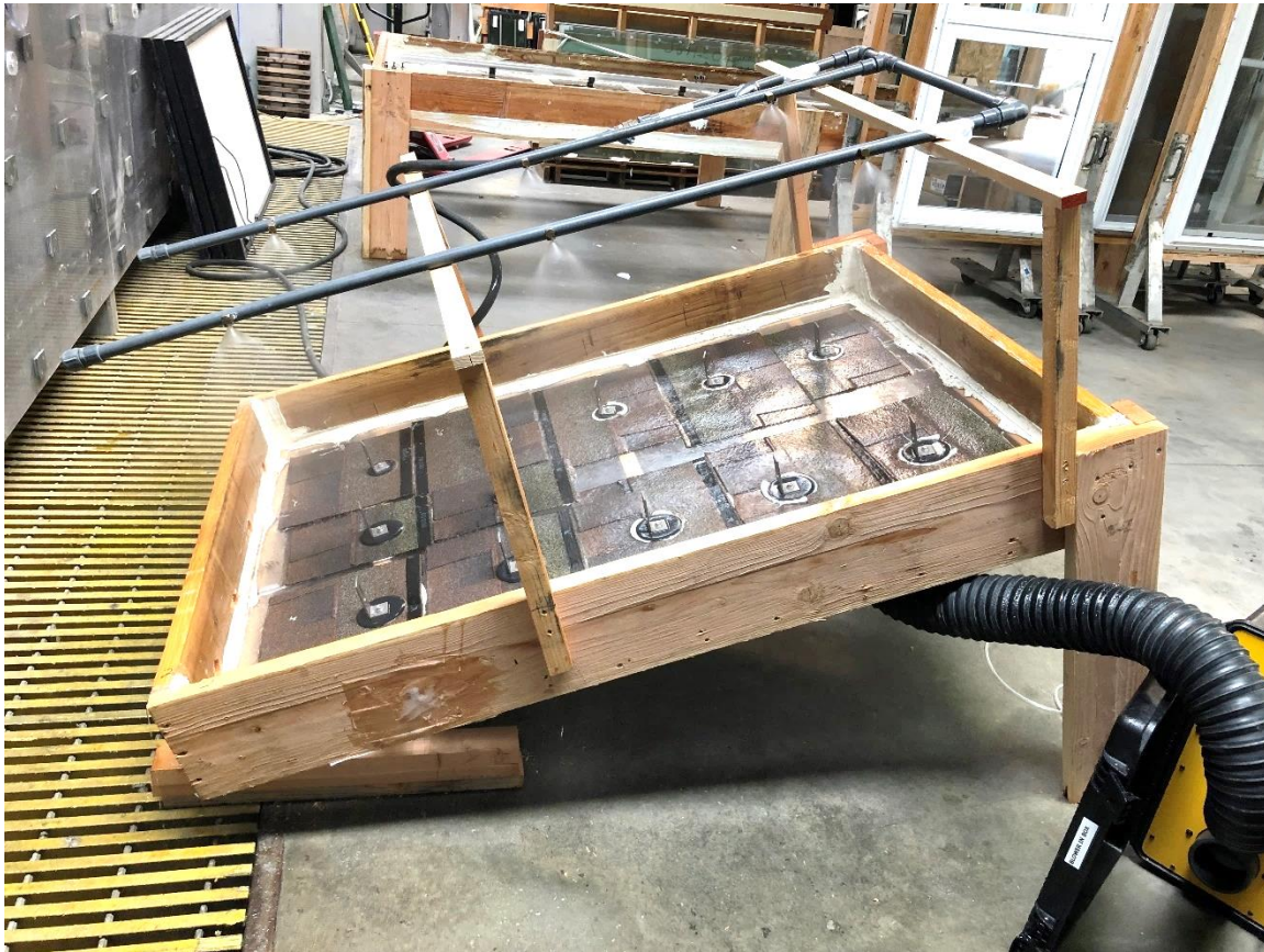
Photo No. 1 The specimen during ASTM E331 testing.
