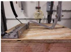
Photo 8: Typical Failure - Contact with Plywood
