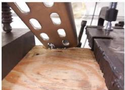
Photo 4: Closeup of Fastener Pullout & Failure
