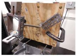
Photo 11: Deformation and Rotation of Hook
