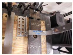
Photo 1: Tensile Test Setup
