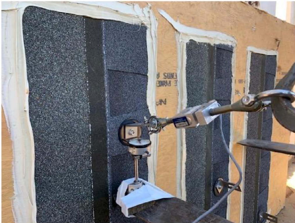
Photo No. 1 Pullout Test
