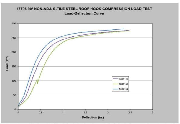
Note: Maximum deflection and peak load taken before sharp increase in load, when hook contacts plywood test board
